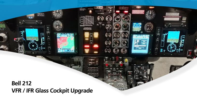
The StandardAero glass cockpit upgrade for the Bell 212 addresses obsolescence challenges with a complete economical solution that brings together proven, high-quality flight displays from Universal Avionics, dual touchscreen navigators and a mandate-compliant ADS-B transponder from Garmin, and a lightweight Attitude Heading Reference System (AHRS) replacement from Rockwell Collins Aerospace.
